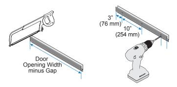
Cut Bottom Adjustment Channel to length. Drill pilot holes every 10" (254 mm) and 3" (76 mm) from each end.
