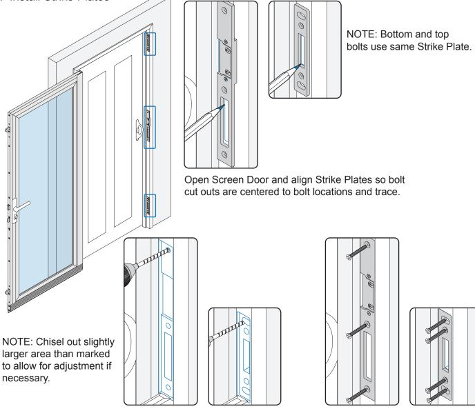
Clean latch hole areas with chisel to accept bolts. Drill 7/64" pilot holes at mounting holes.
